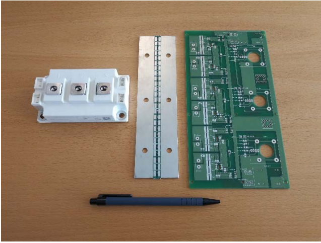
Figure 1: MOSFET power module MD1026HFM150C2S from STARPOWER, capacitor PCB and driver & measurement PCB.
