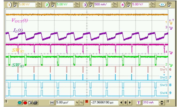
Fig. 5, V_{IN}=3.6V , V_{OUT}=3.3V , RS step-down mode. Ch1: Output voltage, V_{OUT} (5 V/div); Ch2: Inductor current, I_L (200m A/div); Ch3: Boost switching node (5V/div); Ch4: Buck switching node, V_{IN} (5 V/div)
