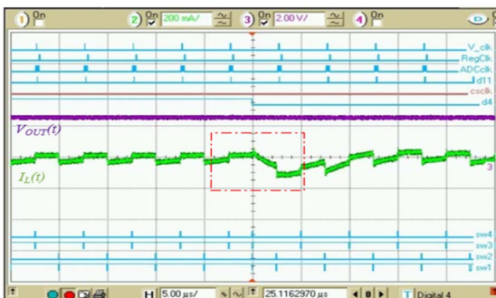
Fig. 11, V_{IN}=3.4V , V_{OUT}=3.3V , Mode transition between Step-down mode and Step-up mode. Ch3: Output voltage, V_{OUT} (5 V/div); Ch2: Inductor current, I_L (200m A/div);
