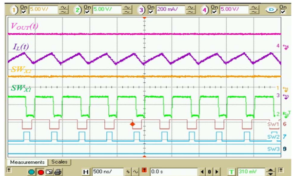
Fig. 7, V_{IN}=2.2V , V_{OUT}=3.3V , Boost mode. Ch1: Output voltage, V_{OUT} (5 V/div); Ch2: Inductor current, I_L (200m A/div); Ch3: Boost switching node (5V/div); Ch4: Buck switching node, V_{IN} (5 V/div)
