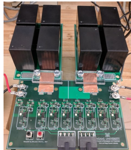
Fig. 5 Modular prototype inverter with two provisional capacitor banks.
