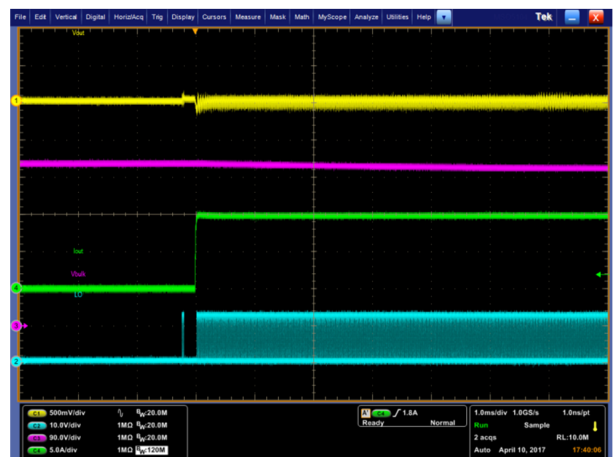
Fig. 12: No load to 10A load transient with the proposed method (Ch1 – Vout AC couple, Ch2 – LO, Ch3 – Vin, Ch4 – Iout)
