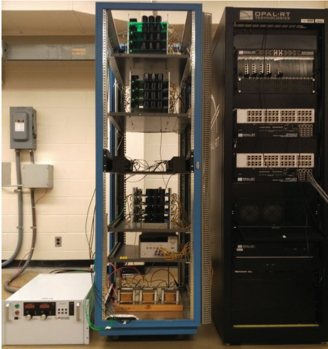
Fig. 5. Experiment Setup of the three-phase MMC prototype.
