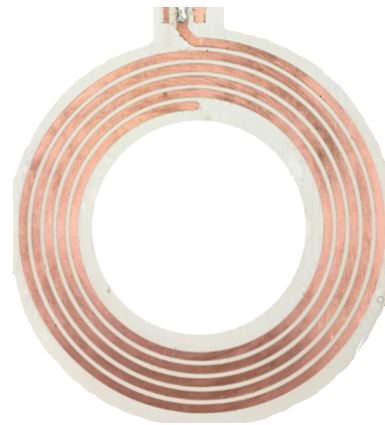
Fig. 15. Self-resonant coil built with RO3003 for further reduced loss.
