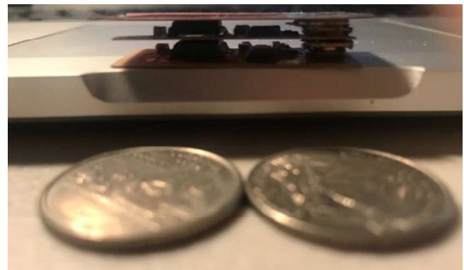
Fig. 4. Assembled 3D 1.2kV SiC half bridge IPM.
