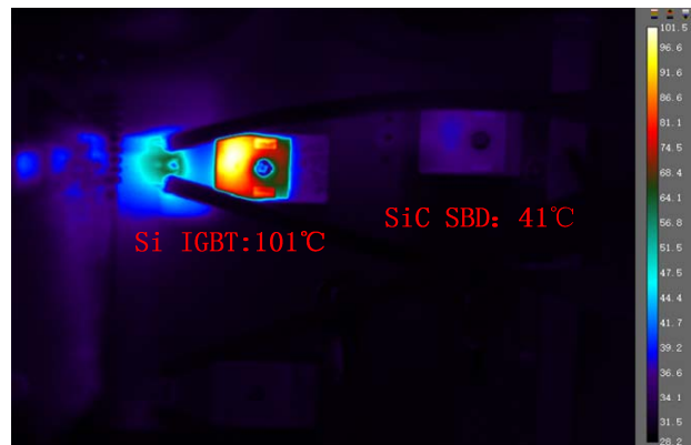
Fig.10: 40A full IGBT 4kw
