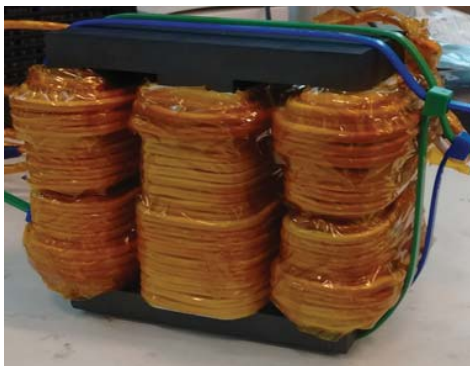
Fig. 9: 10kW/50kHz Three Port Transformer
