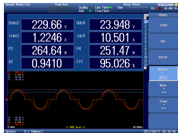
Fig. 9. Line voltage (red), line current (yellow), output voltage (blue) and output current (purple) for the following operating point: input of 230 Vac output voltage of 24 V and output power of 251 W. The power factor is 0.941 and efficiency 95.02%. The line current follows the line voltage.
