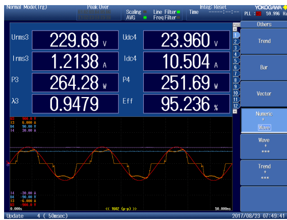
Fig. 11. Line voltage (red), line current (yellow), output voltage (blue) and output current (purple) for the following operating point: input of 230 Vac output voltage of 24 V and output power of 251 W. The power factor is 0.948 and efficiency 95.236%. This data point is taken including all the software changes that increase efficiency. The converter does not draw peak current when the voltage is maximum.
