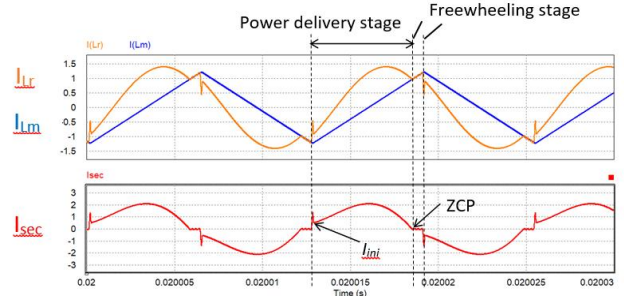
Fig. 7. Simulated steady-state current waveforms of LLC converter without SR ( f_s < f_r ).
