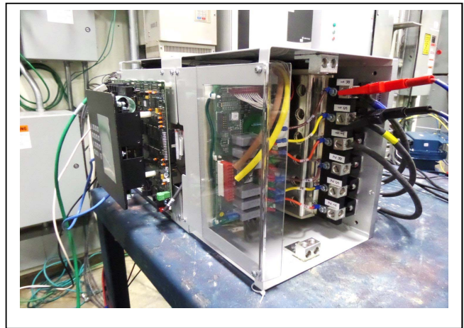
Fig. 22. Experimental of 50HP VFD sample A
