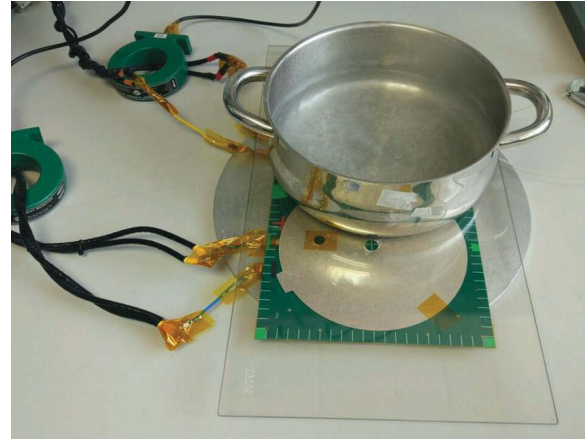
Fig. 9. Picture of the induction load composed of two partially overlapped PCB inductors and a ferromagnetic pot.
