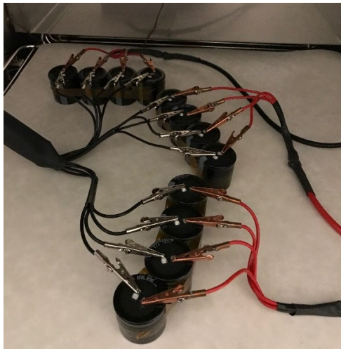
Fig. 8. Capacitor Samples under rated voltage and rated ripple current, placed in a thermal chamber to provide rated ambient temperature.
