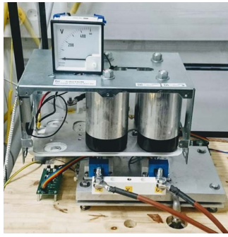
Fig. 3. Two-level single-phase DC/AC inverter
