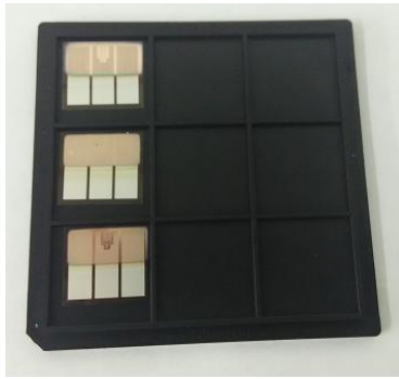
Fig. 8. IGBT die top surface reprocessed with Cu.
