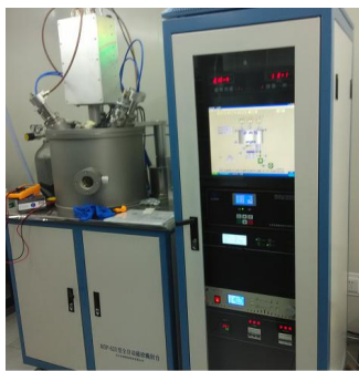
Fig. 5. Sputtering machine for die top surface reprocessing.
