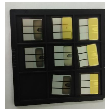
Fig. 7. Diode and IGBT reprocessed with Ti-Ni-Au.
