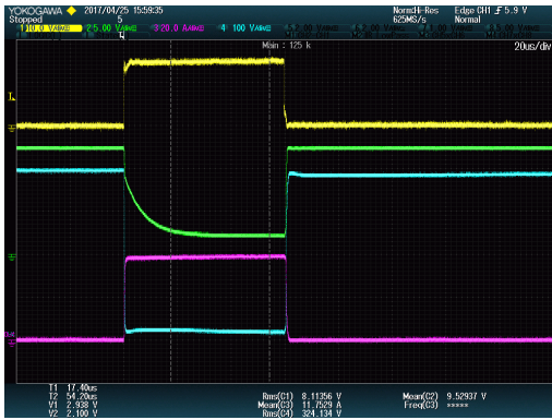
Fig.6. On-state voltage measurement waveforms (400V/40A)
