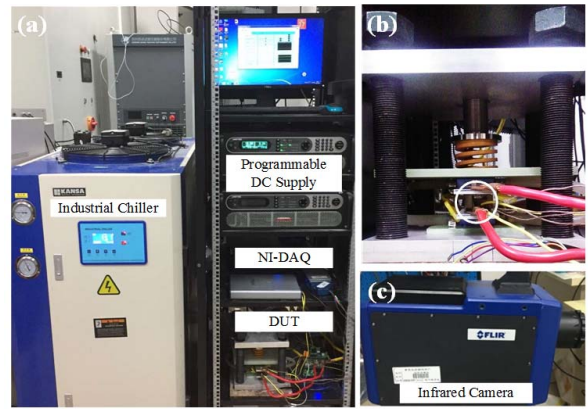
(a) Test vehicle of power cycling (b) Measurement Fixture (c) Infrared Camera
