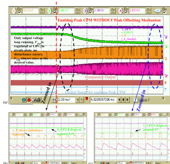
Fig. 8 V_{Cfly} runaway condition in conventional Peak CPM on a three-level buck converter for L = 1.2\mu\text{H} , C = 80\mu\text{F} , C_{Fly} = 75\mu\text{F} , f_{sw} = 500\text{ kHz} , V_{in}(\text{nominal}) = 12\text{ V} , V_{Cfly}(\text{nominal}) = 6\text{ V} , V_{out} = 1.8\text{ V} , D = 0.15 . (a) View of V_{Cfly} drifting in conventional Peak CPM. Time scale: 2 [ms]/div; at trigger point which is three horizontal divisions from the left, conventional Peak CPM is enabled. (b) shows zoomed-in view right after trigger point and (c) shows zoomed-in view of steady-state after trigger point; both (b) and (c) have time scale: 1[ \mu\text{s} ]/div; Ch1. 10[V]/div: V_x ; Ch2. 5[V]/div: V_{Cfly} ; Ch3. 2[V]/div: V_{out} ; Ch4. 2[V]/div: i_{L\_Sensed} .
