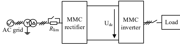
Fig. 6. Two-terminal MMC-HVDC system
