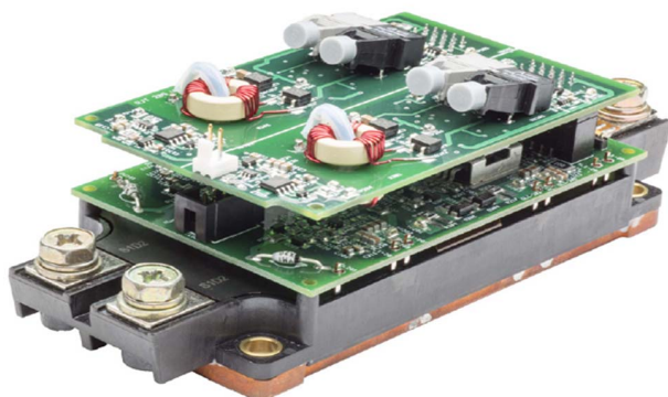
Fig. 1 A 1.7 kV, 450 A Low Inductance GE- SiC MOSFET module from GE with smart gate drive and interface board on top
