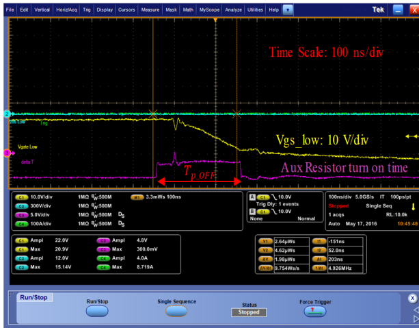
Fig. 14 Implemented T_{p\_OFF} time during turn OFF
