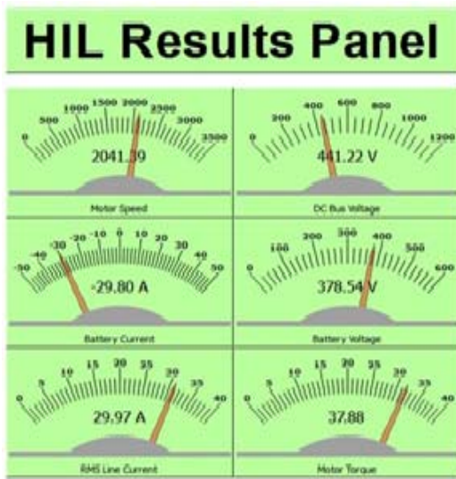
Fig. 10. Motor speed, DC bus voltage, Battery current, Battery voltage, RMS of the motor line current, and motor torque obtained in real-time HIL simulation after 5 secs.
