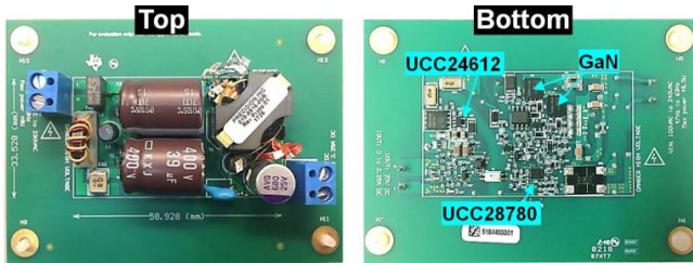
Fig. 11. UCC28780 evaluation board as the GaN-based ACF hardware
