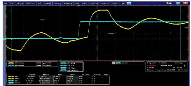
Fig. 7: Drive and motor voltage with 2nd switching instant aligned to zero crossing of motor voltage waveform (DC bus voltage = 610VDC, peak motor voltage = 1064V, ratio = 1.74)
