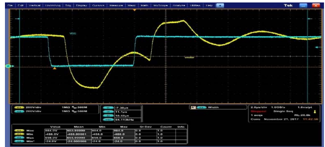
Fig. 6: Drive and motor voltage with 2nd switching instant aligned to positive peak of motor voltage waveform (DC bus voltage = 610VDC, peak motor voltage = 984V, ratio = 1.61)
