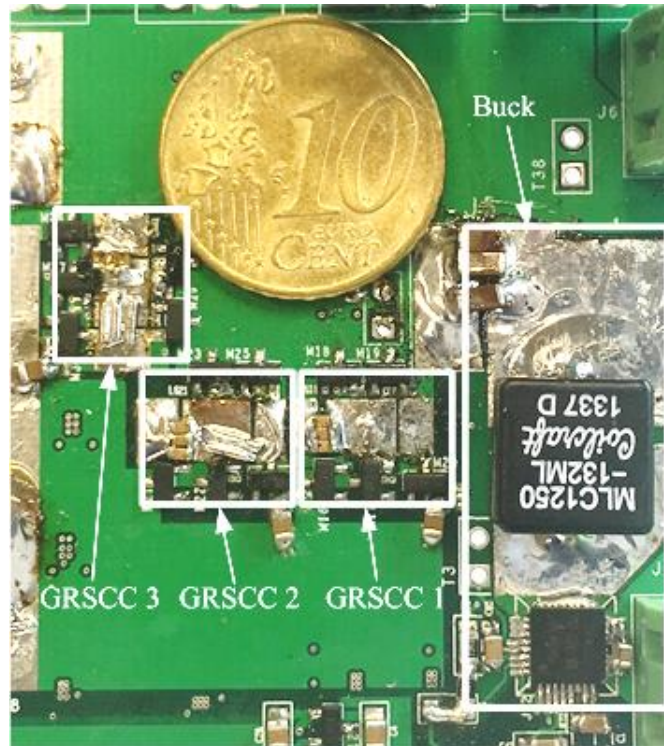
Fig. 50 Photograph of the hybrid-VRM power stage, including the buck converter and three interleaved GRSCCs.
