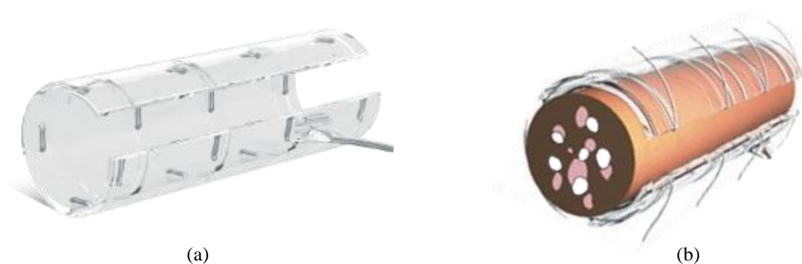
Fig. 1.1 Standard nerve cuff electrode. (a) Typical nerve cuff electrode. (b) Illustration of nerve cuff electrode with peripheral nerve
