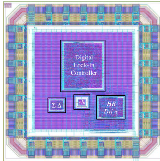
Fig. 4.11 Layout of the fabricated RSCC controller IC.
