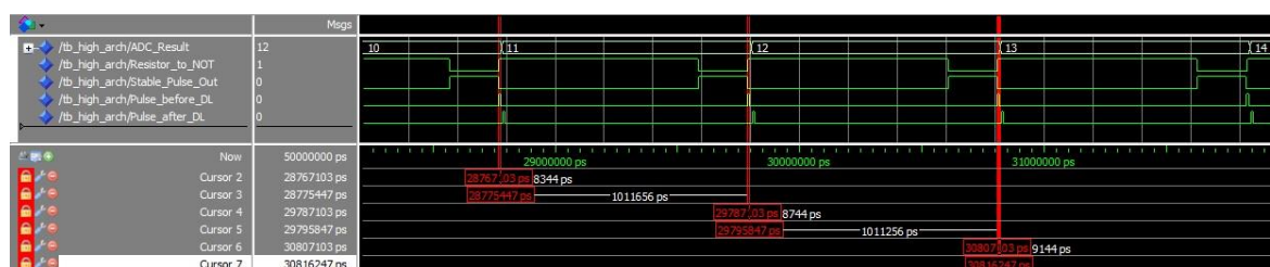
Fig. 3.18 Zoomed results of window ADC – gate level simulation
