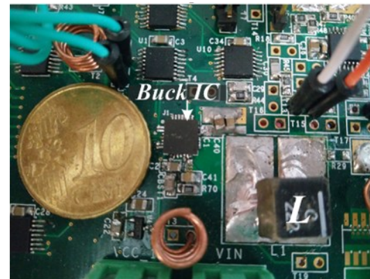
Fig. 9 (a) Micrograph of the fabricated fully-integrated digital average current-mode control 12V-to-1.xV voltage regulator module IC, (b) Chip prototype on PCB.
