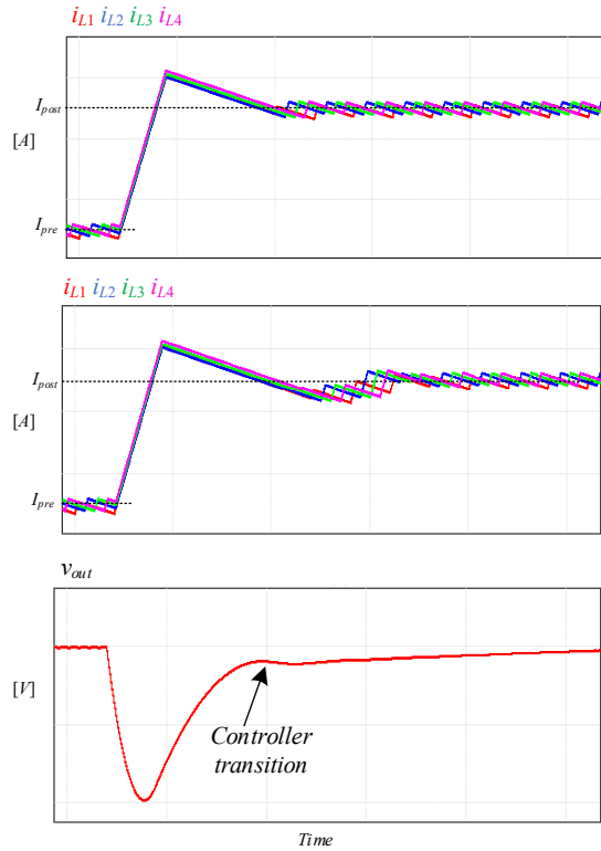
Fig. 8. Hand-off procedure after a loading event for a 4-phase converter. (a) Inductor currents in case the internal and external control signals are compensated. (b) Inductor current without post-transient modifications of the control signals. (c) Output voltage for the implemented hand-off procedure (red) and for the uncompensated procedure (blue).
