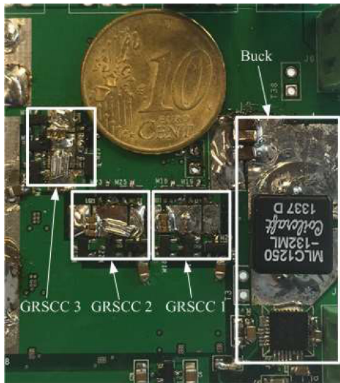
Fig. 12. Photograph of the hybrid-VRM power stage, including the buck converter and three interleaved GRSCCs.
