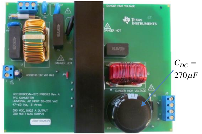
Fig. 7. UCC28180EVM-573 Power Factor Correction Rectifier board.
