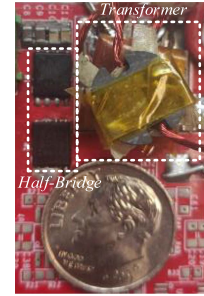
Fig. 16. HB-LLC converter power-stage transistors and transformer.
